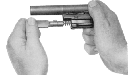
Fig. 39 Extracting the locking piece, firing pin and firing pin spring
