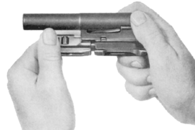
Fig. 38 Stripping the bolt assembly
