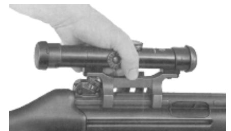
Fig. 55 Removing the telescopic sight with mount
