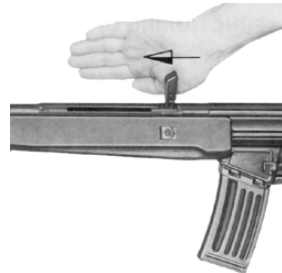
Fig. 33 Releasing the cocking lever
